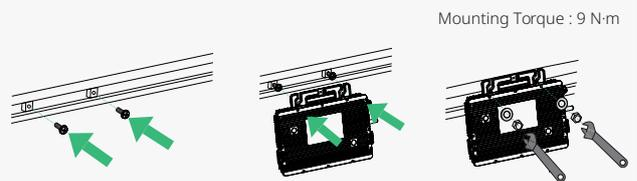
The AC cable contains earth wire, so grounding can be done directly with it. For regions that have special requirements, we offer optional grounding brackets that can be used to complete the external grounding.
