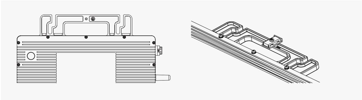
Route a continuous grounding cable through grounding brackets for each microinverter to the AC grounding electrode that conforms with local regulations.
