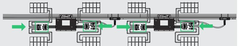
Note: Please use the DC extension cable when the length of DC cable is insufficient to reach the desired location.
